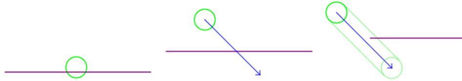
**Figure 6.** The green circle is intersecting with the line in the left diagram, while in the center diagram, the path of the circle intersects with the line. Lastly, in the right diagram, the area swept by the circle intersects with the line.
