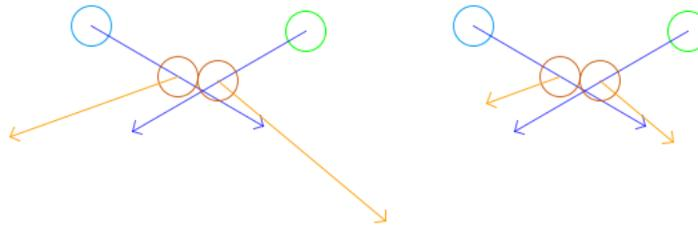
**Figure 4.** On the left is a perfectly elastic collision; on the right is an inelastic collision with a coefficient of restitution of .5. As a result, the resultant vector lines represented by the orange arrows are shorter in the collision on the right.
