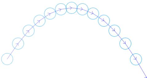
**Figure 1.** The movement of the circle is split up into discrete positions and velocities at certain times (increasing opacity indicates the passage of time), approximating a continuous parametric function, a parabola in this case.
