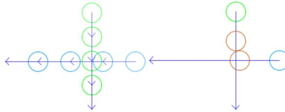
**Figure 2.** Diagrams generated by the collision detection algorithm discussed later in this paper, showing the results of two different collision methods. On the left, the objects are moved forward in small increments and intersections are only done between the final positions, resulting in tunneling. On the right, the collision is detected (in orange) when collision detection is done before the collision occurs
