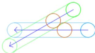
**Figure 3.** The green and blue circles sweep an area as they move along their movement vector. The overlapping of indicates that there is a possibility of a collision occurring between the two circles.
